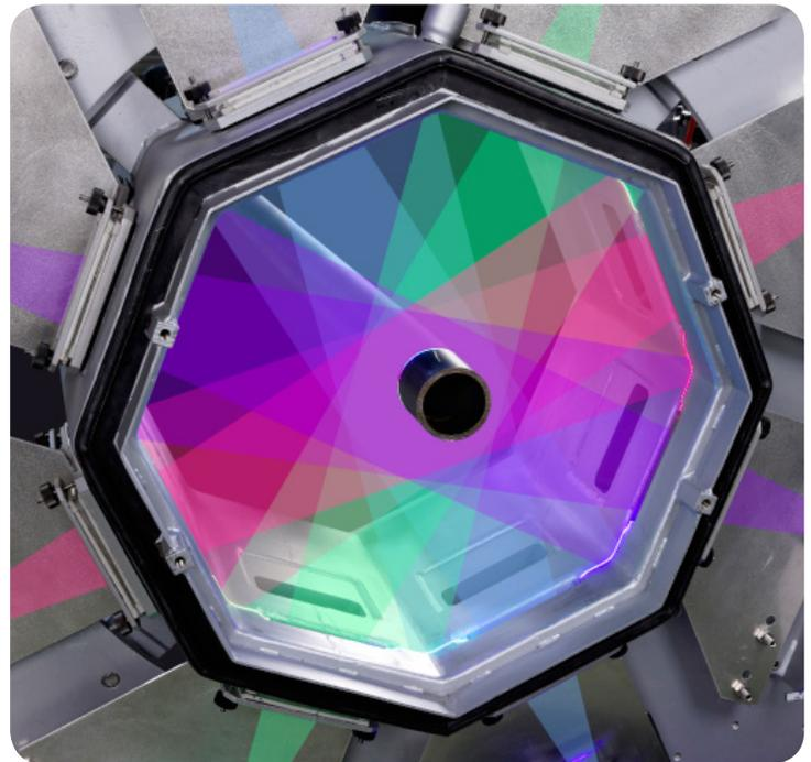
The suitable number of laser camera systems needed for complete and simultaneous measurement of the product is arranged around the periphery. Four to eight sets are typically used, depending on the complexity of the product and the necessary performance. The minimum and maximum product dimensions are also taken into consideration.
